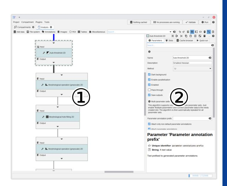
JIPipe comes with its own graphical user interface that allows easy access to all functions. ① The graph editor to build the flow chart ② All settings are shown on the right-hand side
